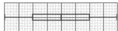
Fig. 3.10. Box plot for a set of data in which Q_3 - Q_2 \approx Q_2 - Q_1 .
